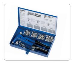
Including threaded mandrels and nosepieces M4 and M6, different blind rivet nut dimensions M4 to M6 made of alu for joint thicknesses of 0.25 to 3 mm.
