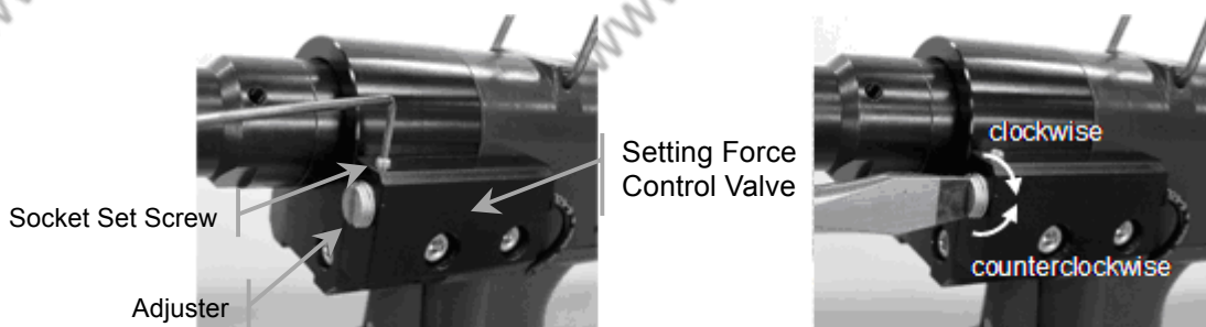
Figure 13: Adjustment of Setting Force
