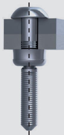
Pintail-less lockbolt after installation
